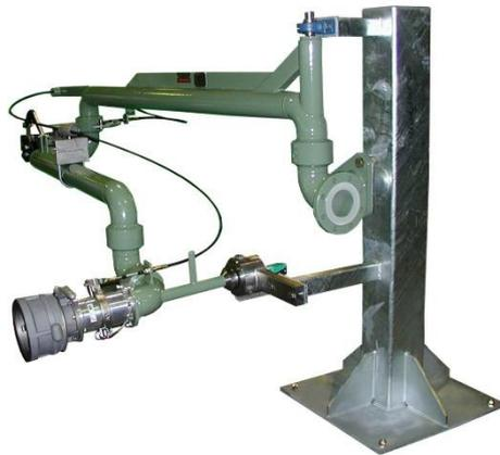
The ERC Release Cable is shorter than a fully extended Loading Arm. This means the ERC will activate and separate before the Loading Arm is fully extended and damaged.
