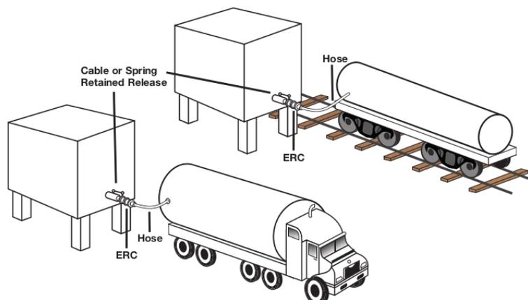
*Shown are conceptual illustrations of typical systems for truck and railcar.*
