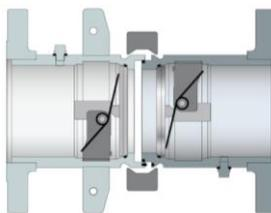
ERC separates allowing the mobile elements of the transfer system to continue in movement without damaging previously connected assets.
