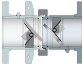
The body seal retains media until the valves close. The media is then contained in both the upstream and downstream sections of the transfer system. The separation sequence continues.
